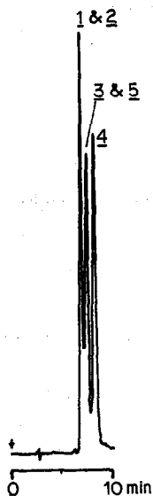
Fig. 2. Normal-phase liquid chromatogram of dppf-substituted metal carbonyls on a Whatman Partisil 5 PAC ( 5\ \mu\text{m} ) column ( 100\ \text{mm} \times 4.6\ \text{mm} I.D.). Mobile phase, isooctane-chloroform (92:8, v/v); flow-rate, 0.5\ \text{ml min}^{-1} ; detection wavelength, 254 nm. Compounds: 1 = (\text{OC})_9\text{Mn}_2(\text{dppf})\text{Cr}(\text{CO})_5 ( k' = 1.49 ); 2 = (\text{OC})_9\text{Mn}_2(\text{dppf})\text{Mo}(\text{CO})_5 ( k' = 1.49 ); 3 = (\text{OC})_9\text{Mn}_2(\text{dppf})\text{W}(\text{CO})_5 ( k' = 1.71 ); 4 = (\text{OC})_9\text{Mn}_2(\text{dppf})\text{Fe}(\text{CO})_4 ( k' = 1.99 ); 5 = (\text{OC})_9\text{Mn}_2(\text{dppf})\text{Mn}_2(\text{CO})_9 ( k' = 1.70 ).
